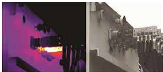
IR problem sample ( Bus termination )
